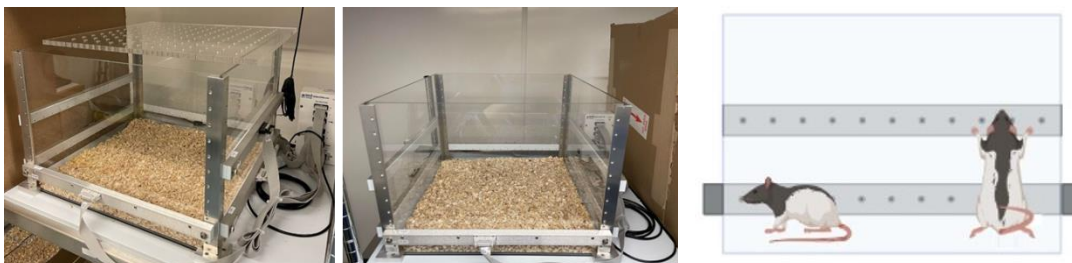
Figure 1: Locomotor activity test boxes and a schematic diagram how the beams record different physical movements of the animal.
